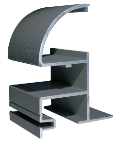
VINYL LINER COPING Top metal bull-nose remains visible; Middle opening receives track; Bottom slot receives vinyl liner edge; Sand infused for easy grip/non-slip
